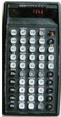
1969: Commodore SR9091SR Texas Instruments chip
