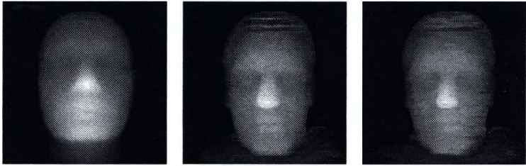
Fig. 10. Disparity Images. From Left to right: synthetic images, normal images with structured light, normal image without structured light
